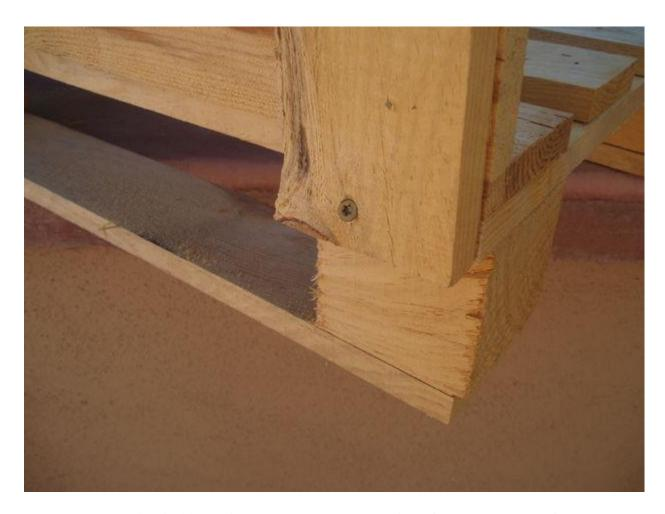
The pallet I am using is  $44 \times 32$  inches. I cut a small portion of the pallet to use for the back rest. With drill/screw gun drive 3, 3 inch screws anchored the back rest to the seat of the bench for support also to hold into place before I get the side supports on. You can use anything for the side supports.
