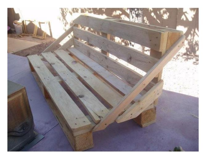
I also found small scrap 2x1 inch wood for side supports. To be honest I held them into place and marked the future pilot holes as well as marked the lines to cut the sides to fit then screwed them into place. I also had a small piece of 1x2-1/2 lumber I used as the bottom support on both sides. You dont have to follow this but I wanted to make sure it wasn't going anywhere. You could also use two pallets lumber to make this bench.
