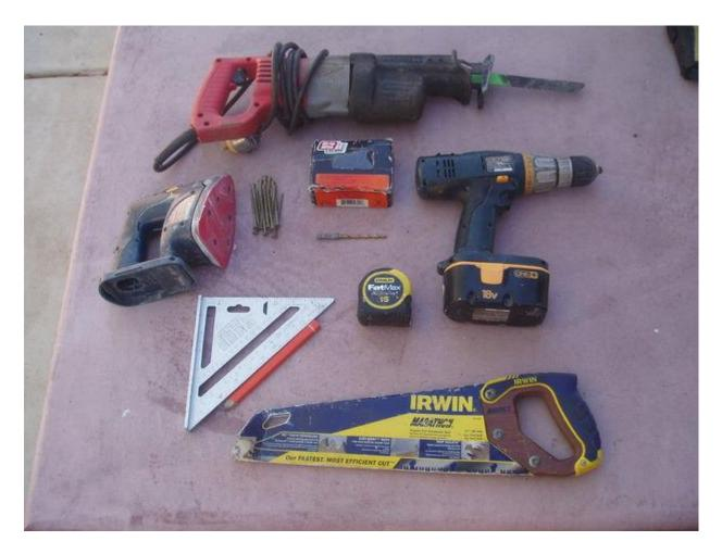
You will need a few tools to get the job done. Drill, drill bit and phllips bit, hand saw (or power saw), 2-1/2 & 3 inch screws, tapemeasure, pencil, square & a sander. I used a 44x32" pallet, a 2x1x36" scrap wood for support& a 7' 2x4 for the legs.
